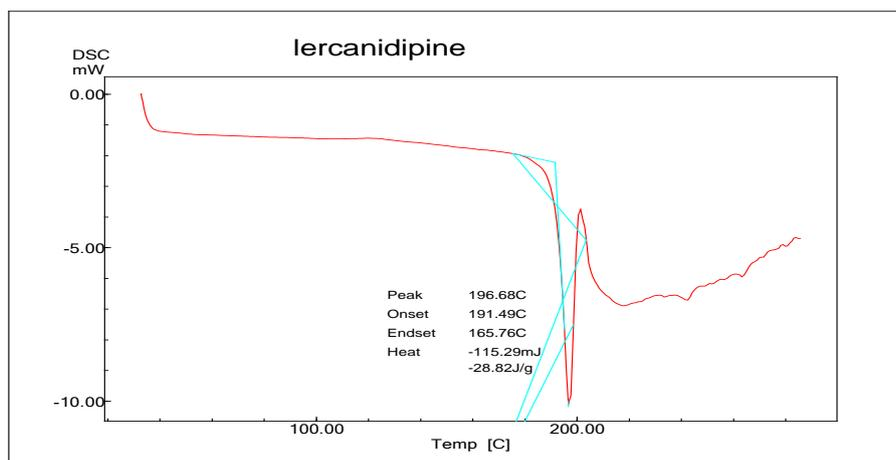
Fig. 2: DSC thermogram of Lercanidipine HCl
