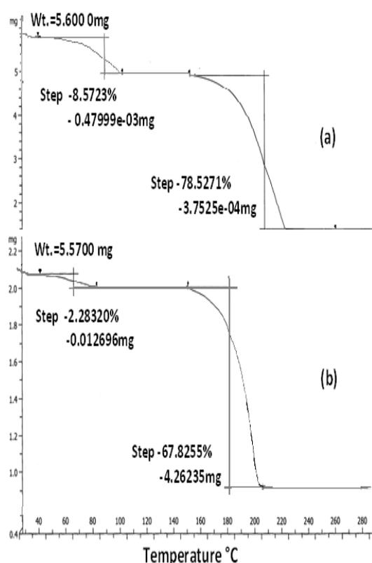
**Fig. 4: TGA thermograms (a) citric acid monohydrate and (b) EFA-CITR**
