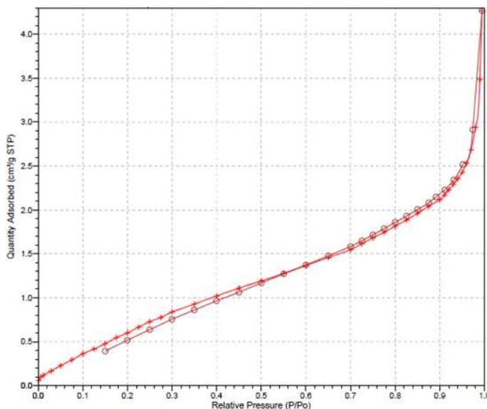
Fig. 5: BET isotherms of [A] intermediate after 1<sup>st</sup> *puta*; [B] final product.
