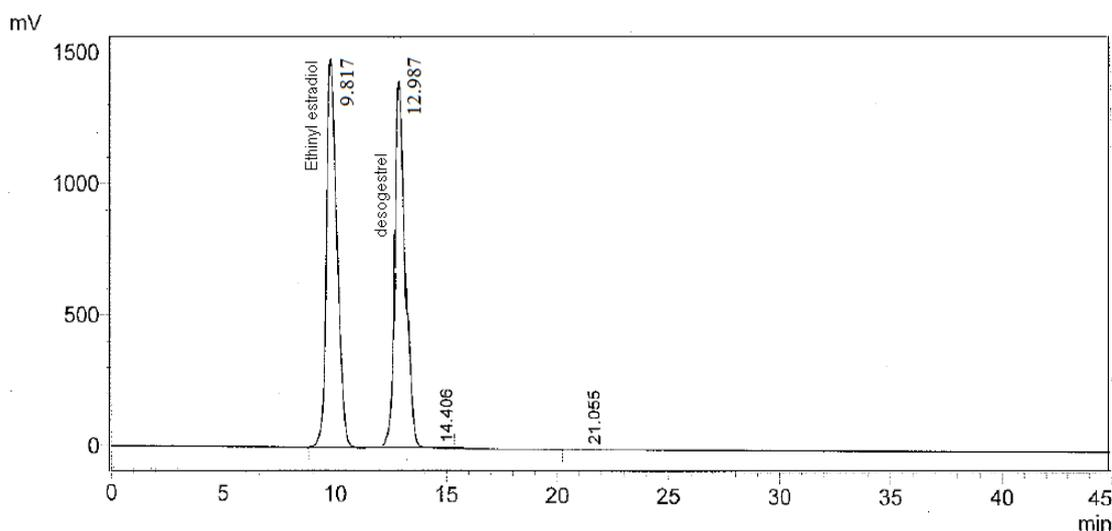
Fig. 4: Chromatographic separation of desogestrel and ethinyl estradiol
