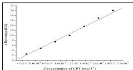
**Fig. 3: Analytical curve for determination of CPT.**
