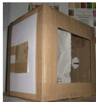
Fig 1: Excito chamber used for mosquito repellency testing
